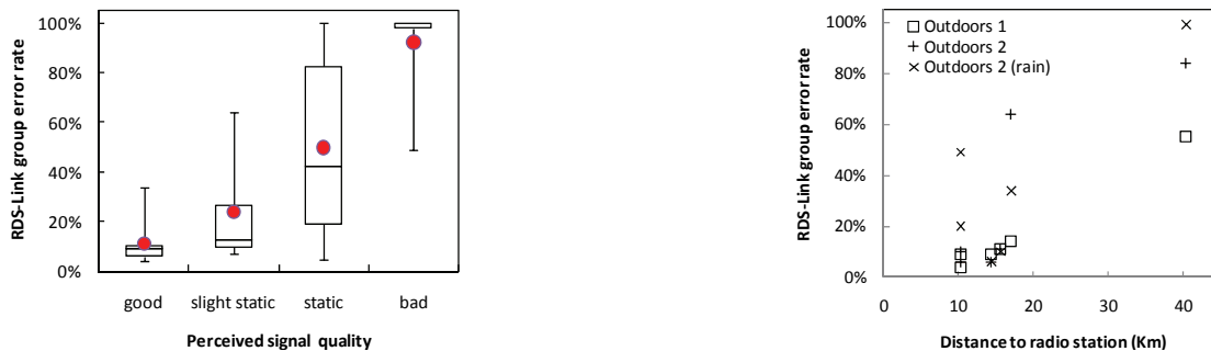
Figure 5. Measured RDS-Link Performance: (Left) Error rate vs. perceived audio quality for indoor and outdoor measurements. Box Plot shows 25 th , 50 th , and 75 th percentiles. Round dots indicate mean, and whiskers indicate maximum values. (Right) Outdoor measured error rates vs. distance from radio stations
